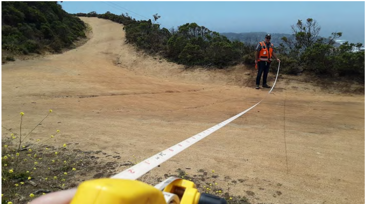
Figure 5: The existing utility clearing at station 81+00 has the dimensions (88' x 34') to be used as a fire turnout.
