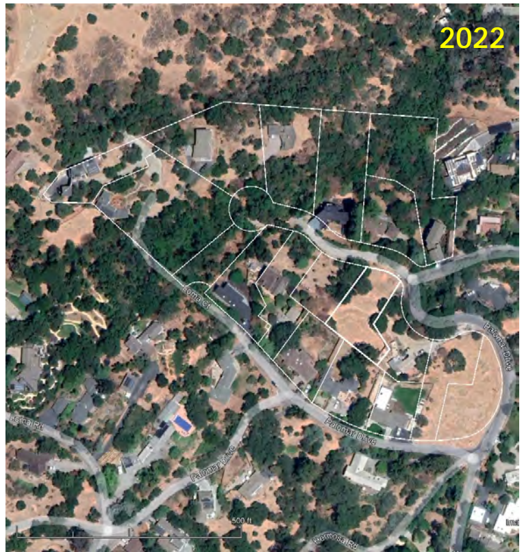
Figure 2. Historical aerial photos show increased home building, tree removal, and landsliding, Los Cerros Rd and Palomar Dr area, San Mateo County, CA. Major landsliding documented during wet years 2017, 1982-83, and 1950s.
