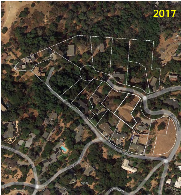
Figure 2. Historical aerial photos show increased home building, tree removal, and landsliding, Los Cerros Rd and Palomar Dr area, San Mateo County, CA. Major landsliding documented during wet years 2017, 1982-83, and 1950s.
