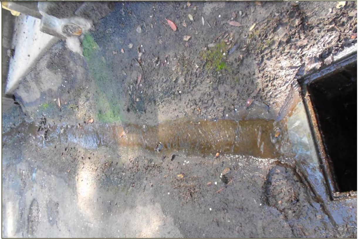
Figure 7. Surface flow on February 13, 2014 near Enea/Charlebois property, APN 051-022-180, Redwood City, California. Surface flow was estimated at less than one gpm at both locations. Water quality samples were collected from both sources (the spring sample from the central portion of the spring).
