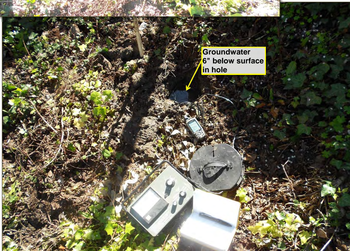
Figure 4. Shallow groundwater on February 13, 2014 at property line of Enea/Charlebois parcel, APN 051-022-180, Redwood City, California. Spring discharge starts just off the photo and near-surface groundwater is found along property line.
