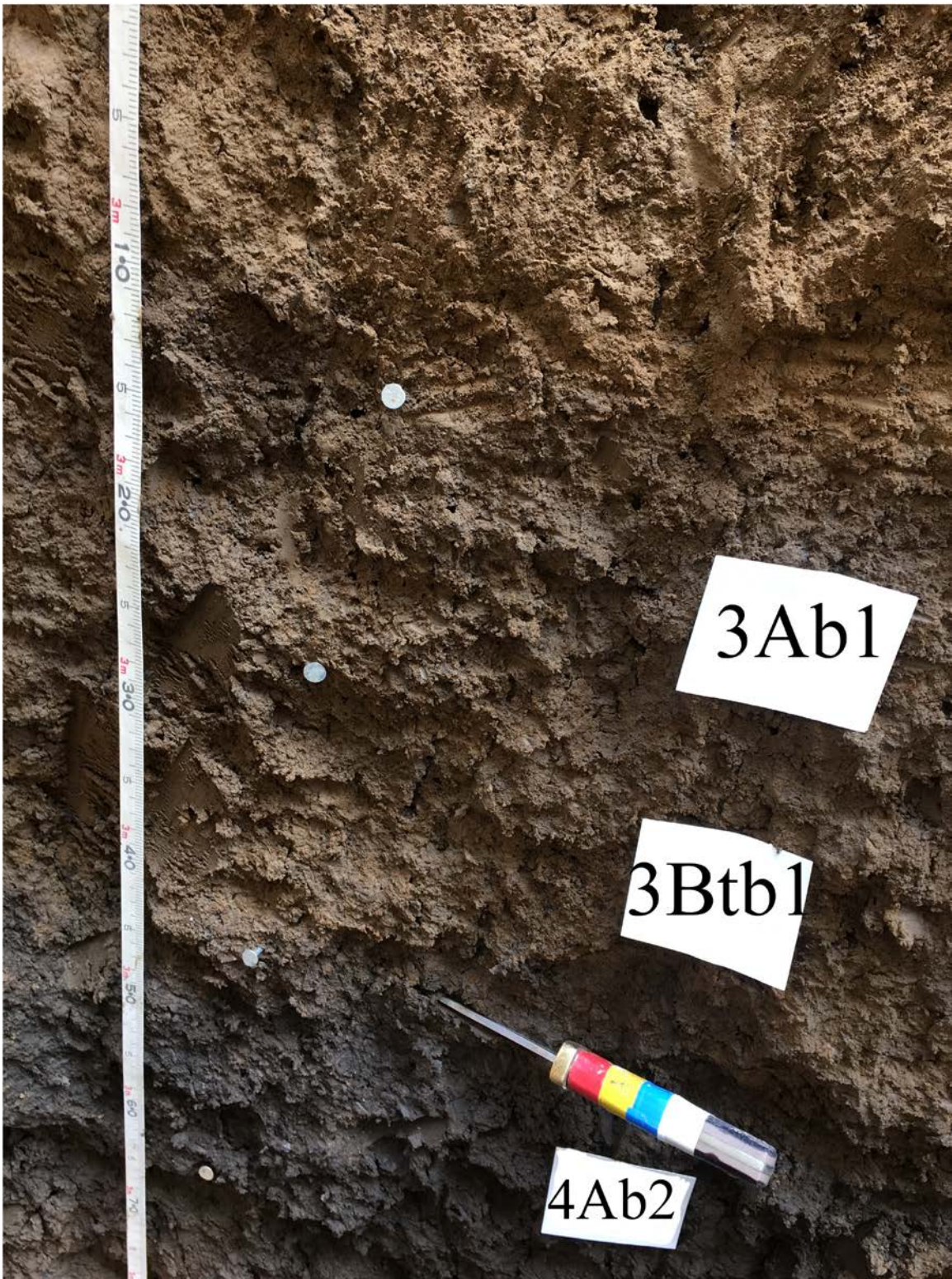
Figure 4. The short-duration b1 and b2 paleosols. The top 1cm of the Ab2 horizon had a C-14 age of 5.3 ka (Table 2). The b2 paleosol was estimated to have a t_d of 1 ka, yielding a t_0 age for the profile of 6.3 ka.
